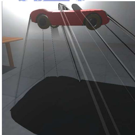
Figure 6.7: Image of car's volumetric shadow. Discontinuous shading problems occur when rendering the shadow of more complex objects. The source of discontinuous shading problems include intersecting shadow polygons, clamping, and perhaps other unforeseen reasons.
