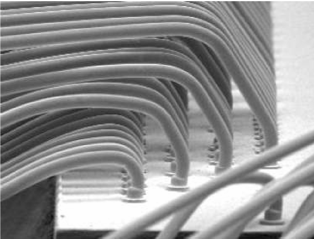
Figure 8. Enlarged image of multi-layered wire bonding (From http://www.kns.com ).
