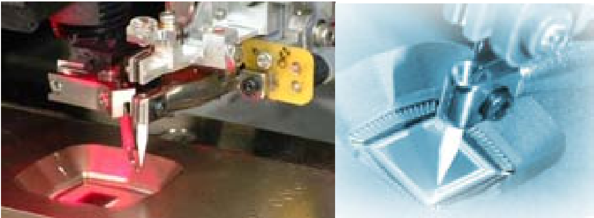
Figure B2. The platen and leadframe in the wire bond working area (From http://www.kns.com ).
