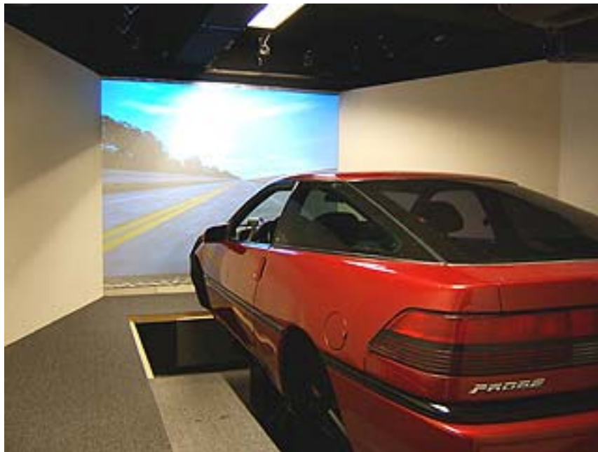
Figure 4-1. The dynamic driving simulation laboratory consists of the virtual-reality-based 360°-surrounding screen and a six-degree-of-freedom motion platform.
