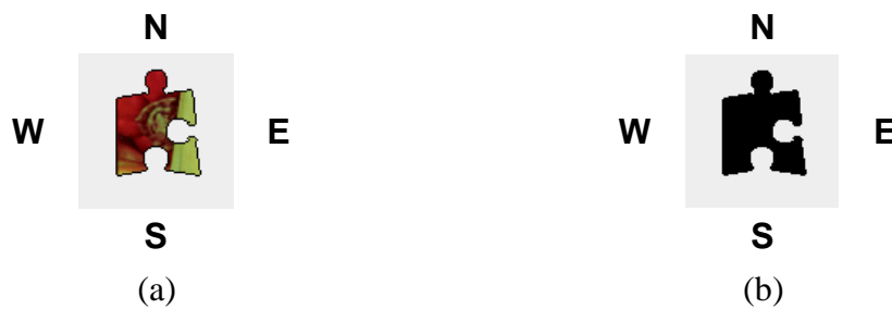
Figure 2.11 An example of a decomposed puzzle piece. (a) N , E , W , and S represent four sides of a digital puzzle piece. (b) The puzzle piece region map ( PM ) derived from (a).
