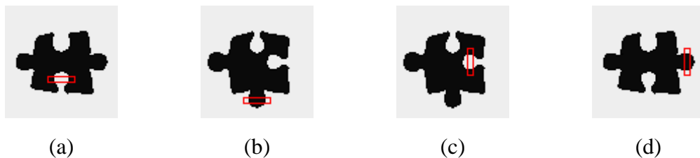
Figure 3.3 Scanning regions of the puzzle piece size detection process are within the red rectangles.
