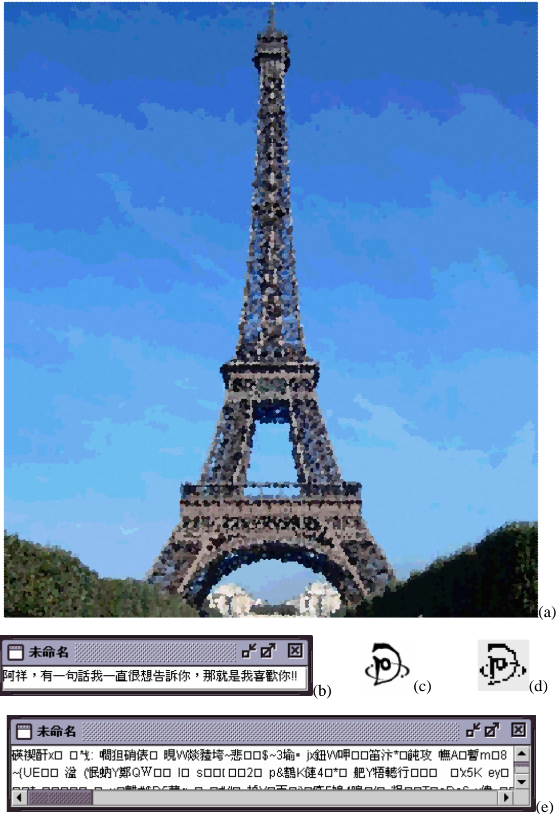
Figure 4.17 Experimental results of secret hiding in a pointillistic image. (Transform an original image into a digital watercolor image first) (a) A pointillistic image with secret message and the watermark, (c), embedded. (b) The secret message extracted from (a) with a correct key. (d) A watermark extracted from (a). (e) The extraction result of (a) with a wrong key.
