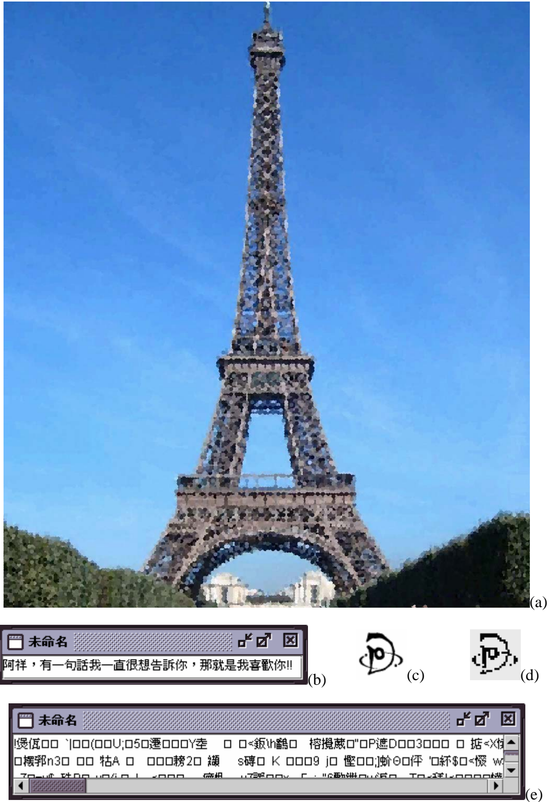
Figure 4.16 Experimental results of secret hiding in a pointillistic image. (a) A pointillistic image with secret message and the watermark, (c), embedded. (b) The secret message extracted from (a) with a correct key. (d) A watermark extracted from (a) with a correct key. (e) The extraction result of (a) with a wrong key.
