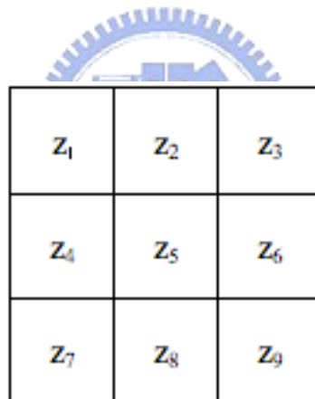
Fig. 2- 2 A 3 \times 3 region of an image (the z 's are gray-level values) used to compute the gradient at point labeled z_5
