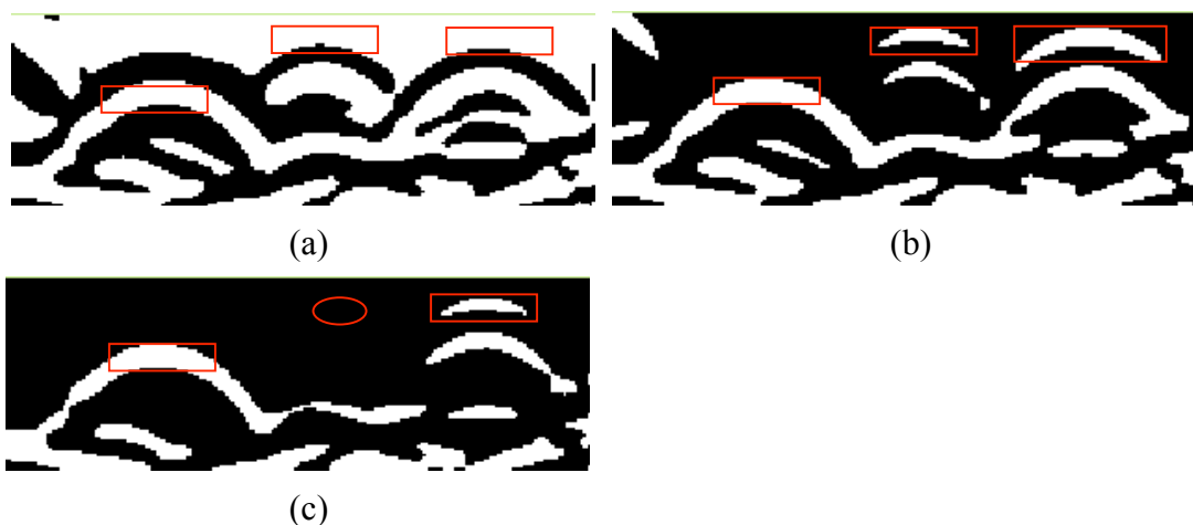
Fig. 3- 6 Binary images for difference hard thresholding value: 128,130,135, and this red circles mean invisible object and the red rectangle mean the object location.
