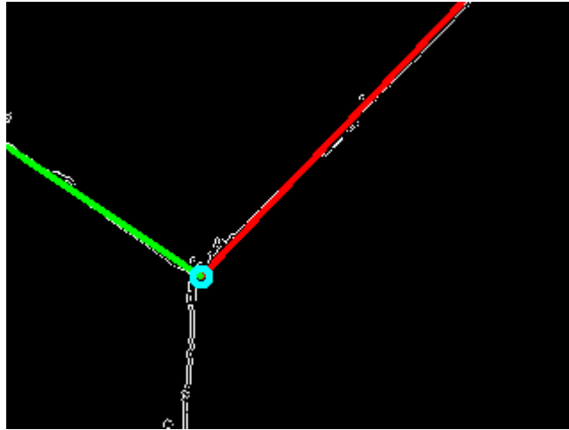
Figure 3.14 Refitting of two non-vertical corner edges.
