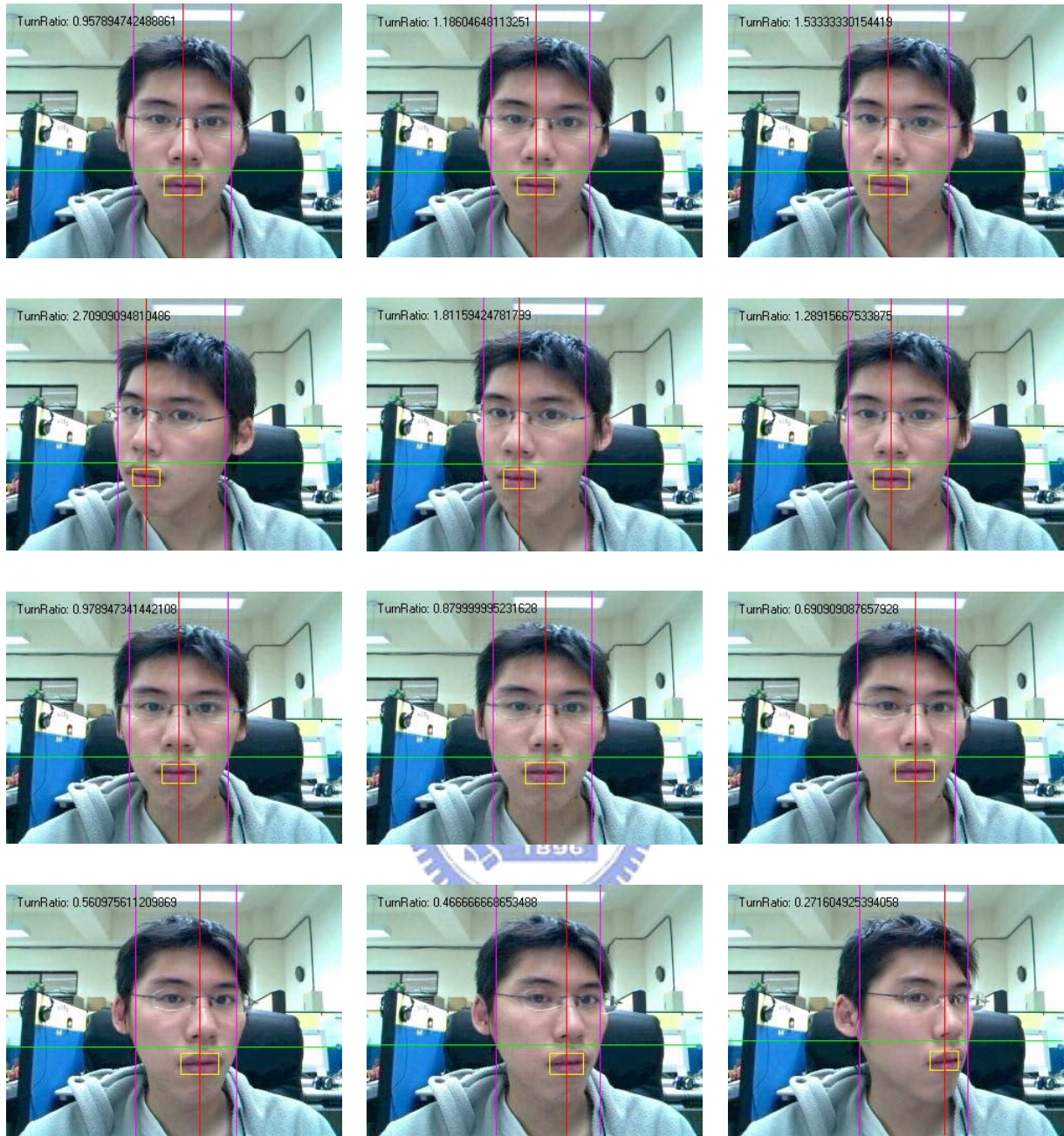
Figure 3.16 An experimental result of detection of head turnings in sequential facial images.
