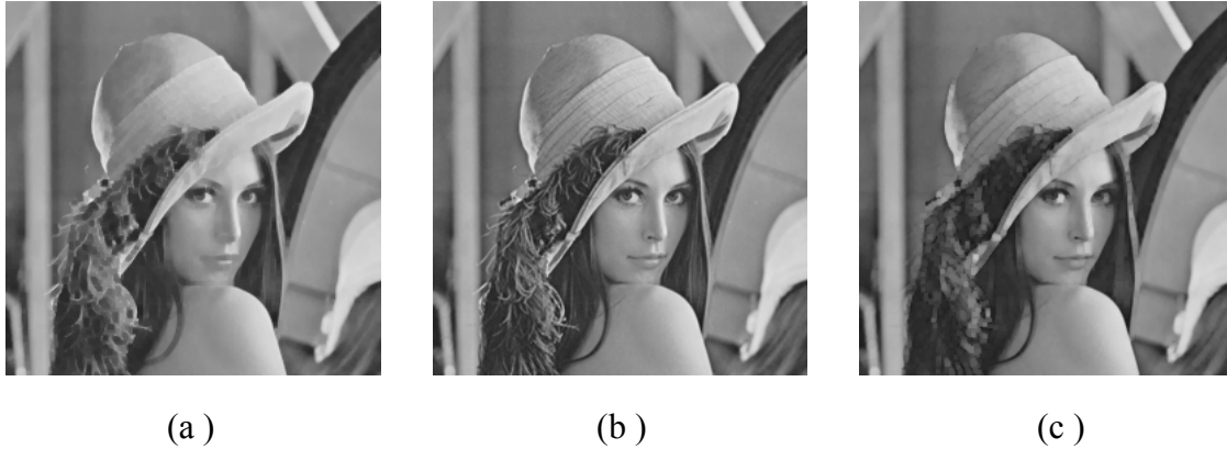
Fig. 2- 20 (a) The original of Lena image (b) Closing of Lena image (c) Opening of Lena image
