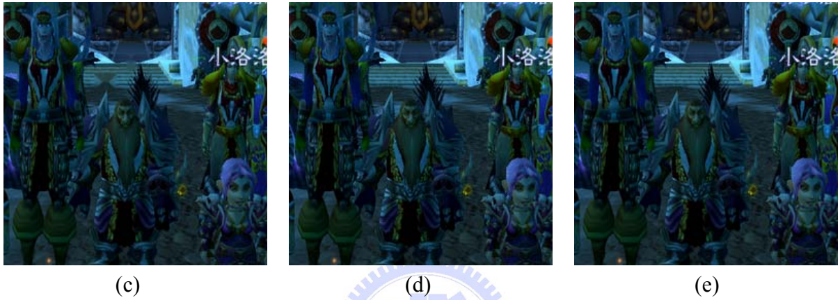
Fig. 4- 11 (a) Original image (b) Damaged image (c) The inpainting result of Fast Digital Image Inpainting; (d) The inpainting result of Priority Texture Synthesis; (e) The inpainting result of the proposed method. Notice the difference in the stairway of the game's image between (a), (c), (d) and (e).
