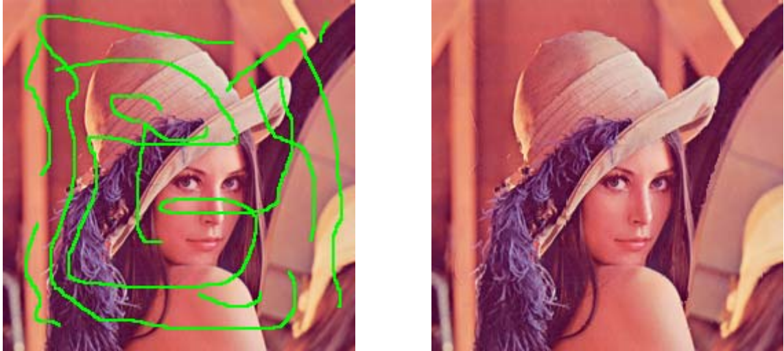
Fig. 2- 5 Lena : (left) Picture with locally small damaged regions. (right) Restored image obtained with fast inpainting algorithm.
