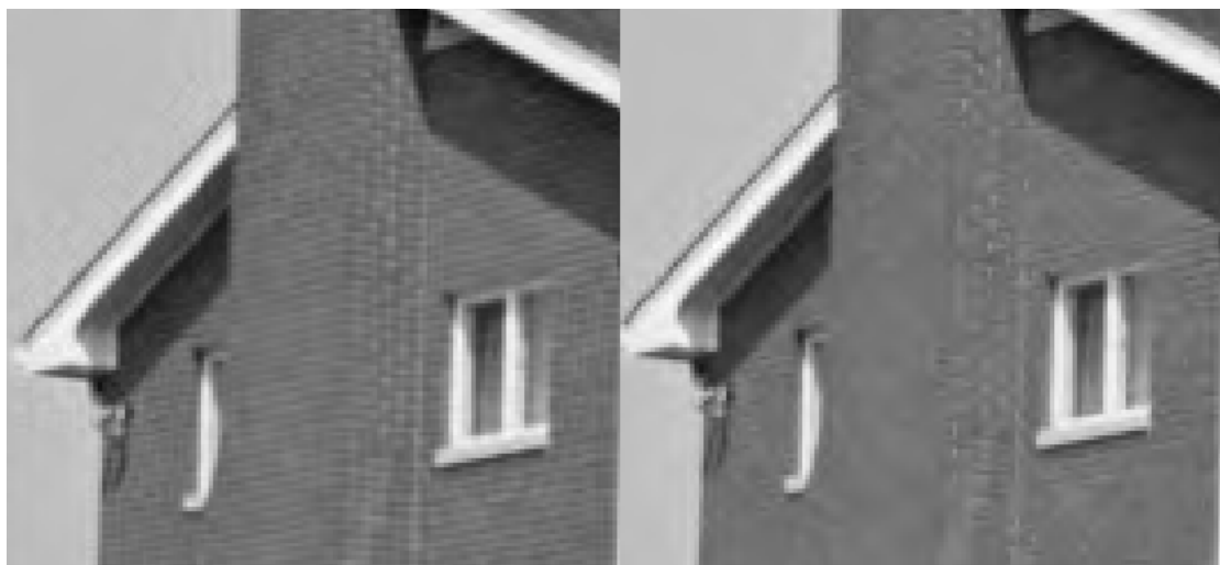
Fig. 4-13. 8-4-2-2-2 DCT (left) V.S. Original SPIHT encoder (right)
