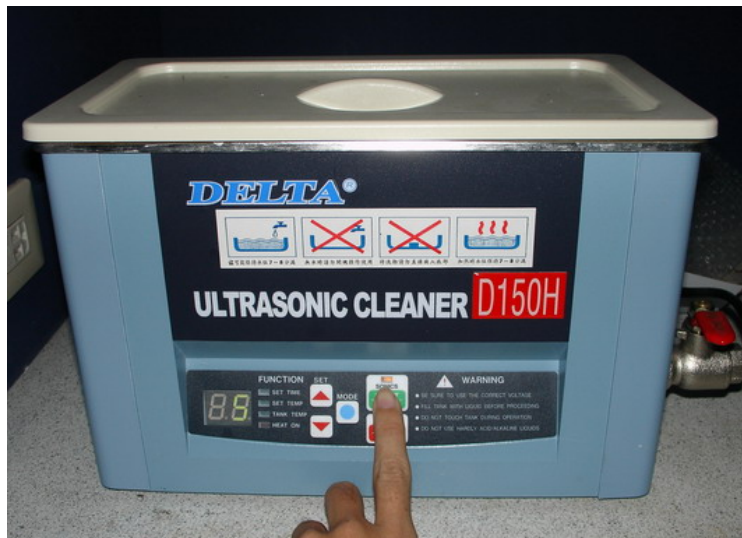
Fig. 3-3. Ultrasonic cleaner for glass substrate cleaning.
