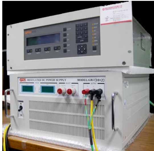
Fig. 3.12. Photograph of pulse DC controller and DC power supply.
