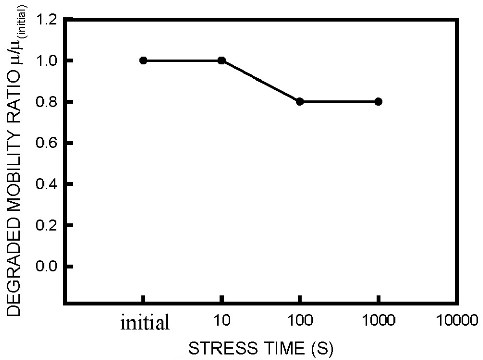
Fig. 4-18 the degraded mobility ratio versus stress time curve of an n-channel ELA TFT with 1.5 \mu\text{m} LDD at V_{DS}=0.1\text{V}
