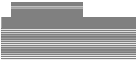
Figure 4.9 1st step of process: mesa
