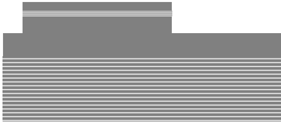
Figure 5.7 1st step of process: mesa
