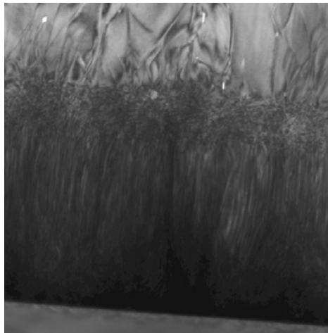
Fig. 5-5 Cross sectional TEM image of a-plane GaN with SLs.
