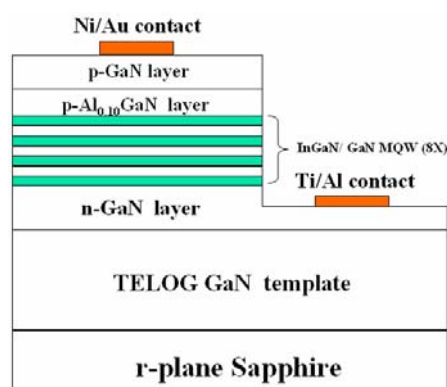
Fig. 7-1 Structure of the ultraviolet nonpolar TELOG LED.
