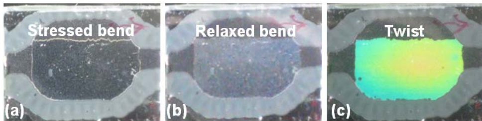
Fig. 4-7 Photographs taken while driving the pi-cell with impulse waveform, where (a) stress bend, (b) relaxed bend, and (c) twist states show full extinction, slight light leakage, and full transmission, respectively.
