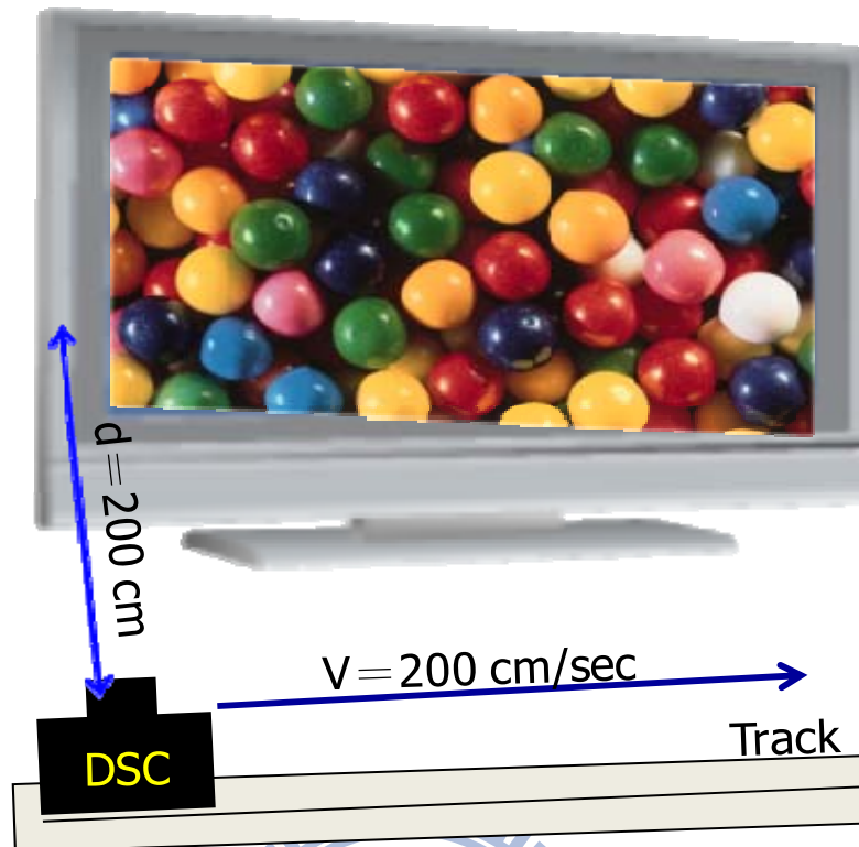
Fig. 4-21 Experimental setup for capturing CBU images.
