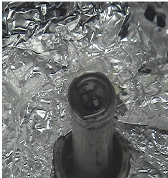
Figure 2.8: Applying some amount of glycol on the TFB layer.
