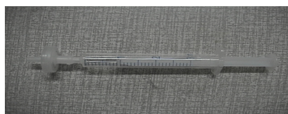
Figure 2.7: The filtering gadget consisting of a PE syringe and a filter.
