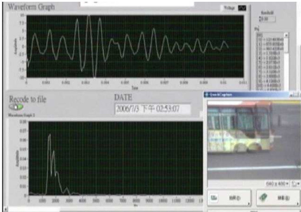
Figure 1.3: The top figure shows the snapshot of the received voltage signals when the bus shown in the image was within the illuminative field of the road-side radar, and the bottom figure shows the frequency-domain frame that is obtained by converting received voltage signals via FFT.
