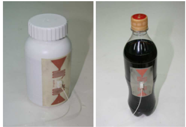
Fig. 6. (a) The RFID tag attached to a vitamin-filled plastic bottle. (b) The RFID tag attached to a liquid-filled plastic bottle.
