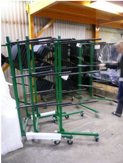
Figure 12) The in-house developed stackable holders with wheel, are very space efficient
