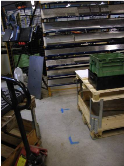
Figure 11) The pallet Kanban system for the welding, marked with blue marks on the floor
