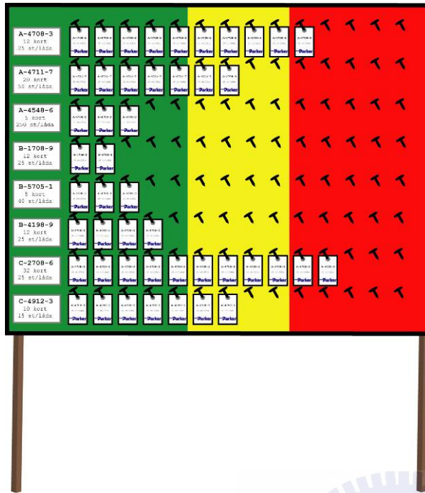
Figure 3) A kanban board, as they look like in Parker Hannifin’s production facilities. (Cameras were not allowed in the factory, so the figure is drawn in Adobe Illustrator by this report’s author)
