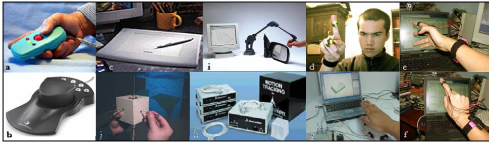
圖1 操作不同類型的輸入工具：a和b為3D滑鼠 ( http://www.3dconnexion.com/products/3a3.php )；c為手寫板；d、e和f為LED手套；g為紅外線定位裝置；h為磁性定位裝置 ( http://www.ascension-tech.com/ )；i為“MicroScribe” ( http://www.immersion.com/digitizer/products/microscribe_g2.php )；j為Cube mouse ( http://imk.gmd.de/docs/ww/ve )
