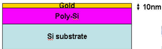
Figure 4.14a Formation of gold silicide at 10nm gold thickness
