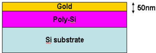
Figure 4.13a Formation of gold silicide at 50nm gold thickness
