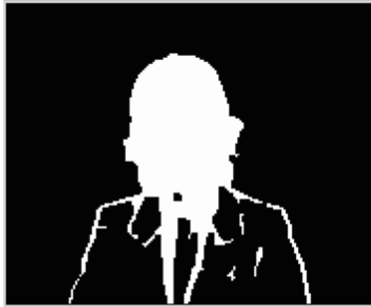
Figure 3.18: Threshold frame difference map after remove small region of frame 60 in Claire sequence.
