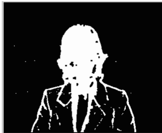
Figure 3.13: Threshold frame difference map of frame 27 in Claire sequence after closing operation.
