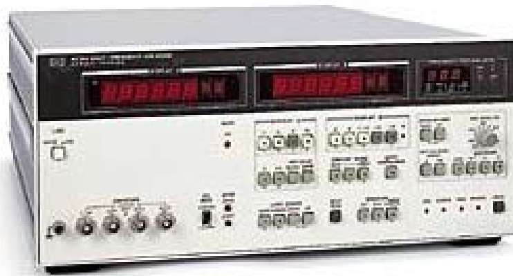
Fig. 3.4 The LCR meter which is used for the measurement of capacitance (Agilent 4275A).
