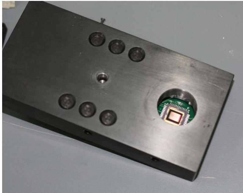
Figure 25: The high-speed CCD sensor -- front view.
