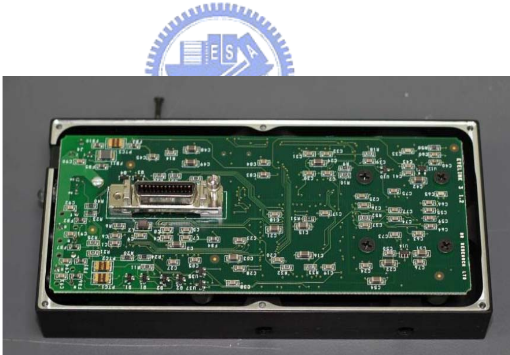
Figure 26: The high-speed camera module -- rear view.
