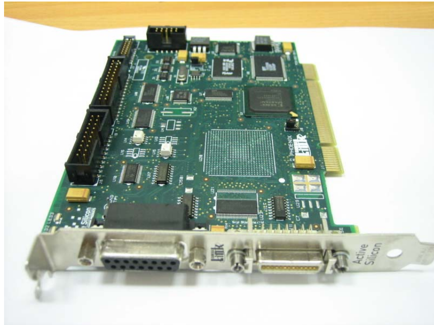
Figure 27: Digital frame grabber for capturing video data.
