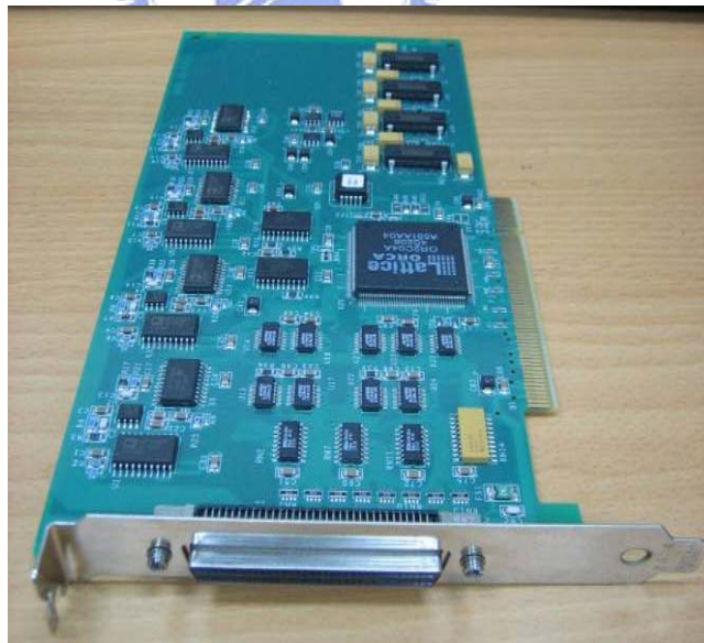
Figure 28: Analog interface card for external communication.
