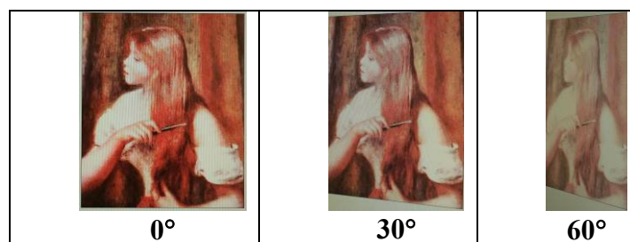
Figure 77: Luminance/contrast degrades and color shifts as viewing angle increases from 0° to 30° and 60° on a 19" TFT-LCD. The extreme angles, which seldom occur in practice, were chosen to emphasize the visual distortion.
