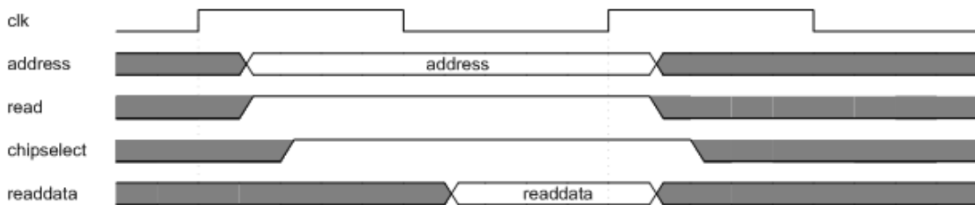
Figure 14: Read protocol of Avalon Bus (wait 1 cycle)
