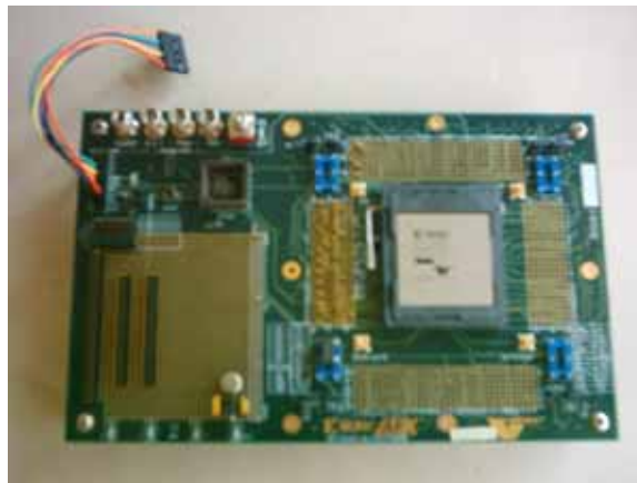
Figure27. Xilinx prototype board with Virtex E FPGA Chip
