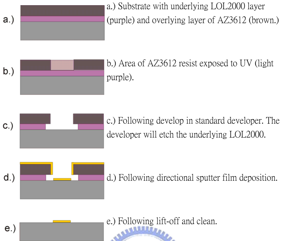
Figure 2-9 The typical lift-off process introduction
