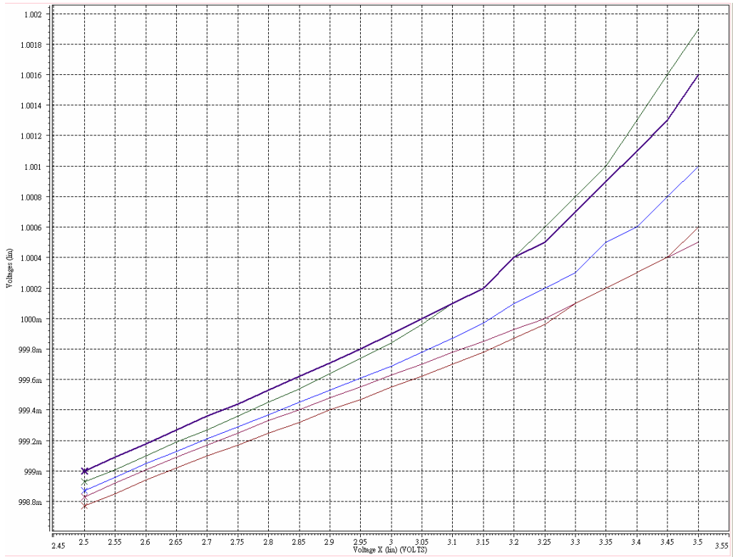
Fig. 3.2-21 Bandgap reference VDDA variation (2.5-3.5V) v.s temperature variation extracted from this thesis' (Shao-Hang Hung. 's ) coordination
