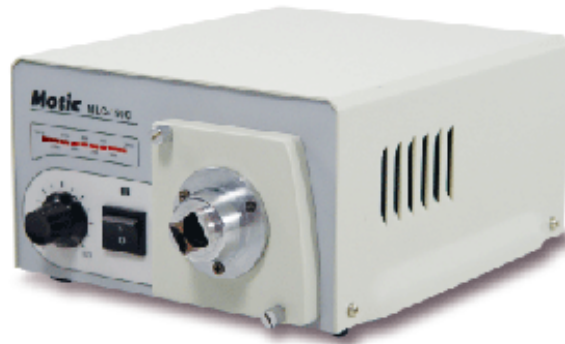
Fig. 4.4-4 Fiber optic illuminator MLC-150C extracted from Motic Cooperation < 10 >
