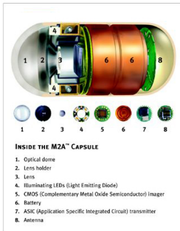
Fig. 5.2-2 Capsule Endoscopy ( a ) Outlook ( b ) Architecture extracted MAYO Clinic Inc. " Capsule Endoscopy", MAYO Clinic Medical Service < 9 >
