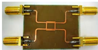
Fig. 3.65. The quadrature hybrid of 7920MHz.
