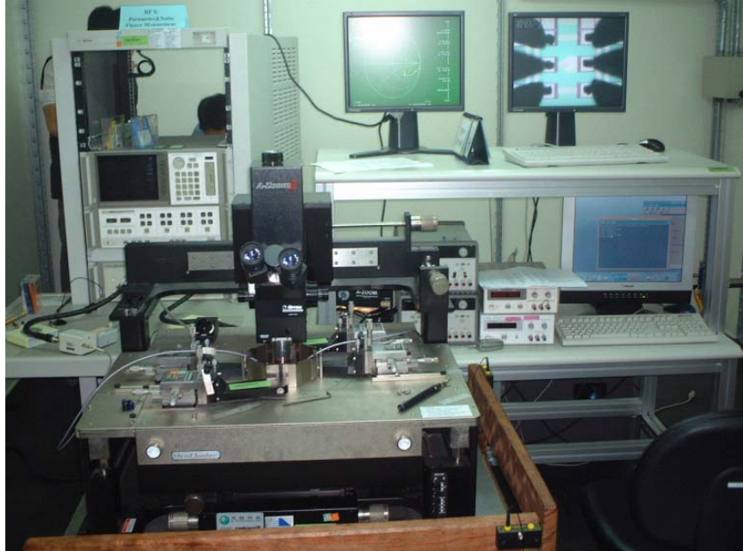
Fig. 3.22 The high frequency S-parameter measurement system.
