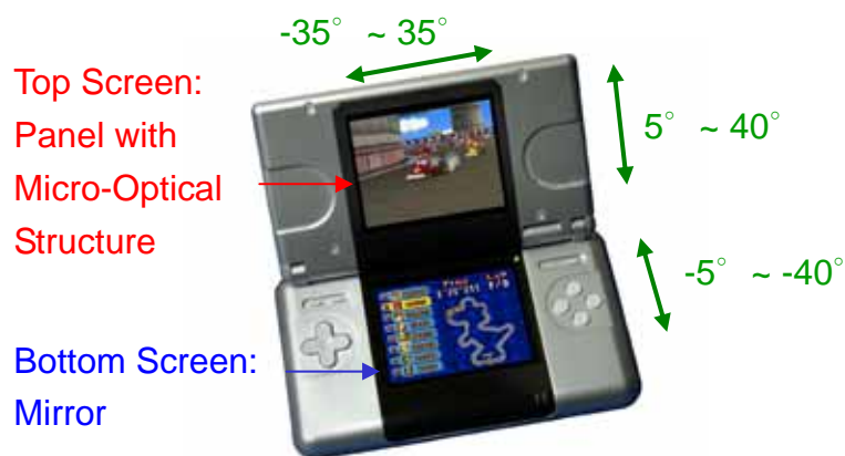
Fig. 3-11. Schematic diagram of acceptable viewing-angles for top and bottom screens.
