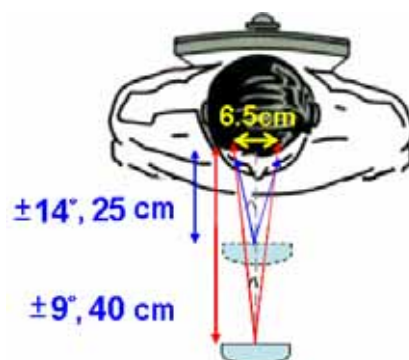
Fig. 3-8. Schematic diagram of viewing angles at near and further viewing positions.
