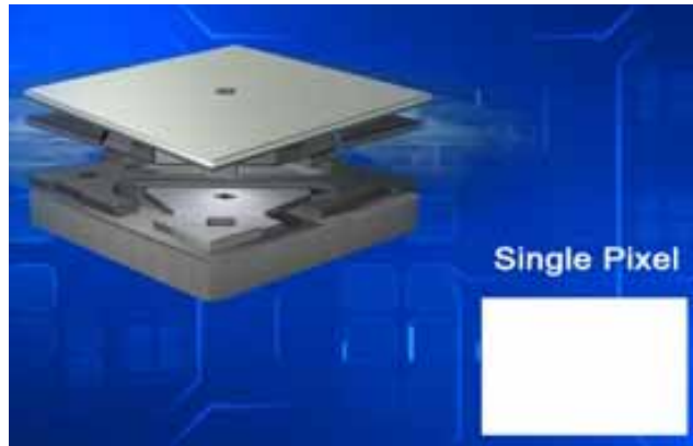
Fig. 3-4. The structure of a single pixel of DMD and the relative light gray pixel.
