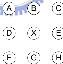
Figure 3.4 – Threshold from Mean of 8 Surrounding Pixels
