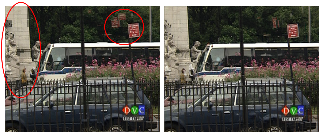
Figure 3-7 The low-pass frame after 4 temporal decompositions: Bus_CIF (Left: without I-Block; right: with I-Block)
