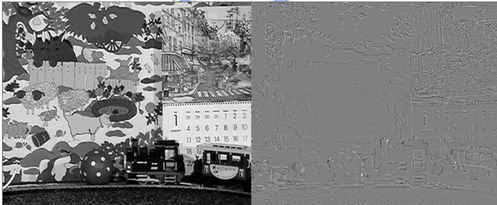
Figure 2-5 Temporal filtered image with motion compensation (Left: low-pass, Right: high-pass)
