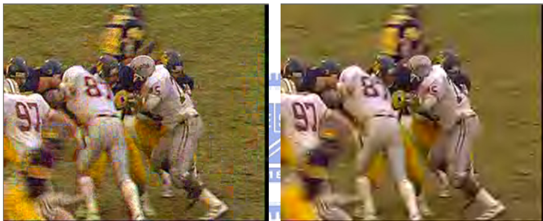
Figure 3-12 Subjective quality comparison of proposed scheme (left) and MC-EZBC (right). (The 39 th frame of Football_CIF at 500kbps.)
