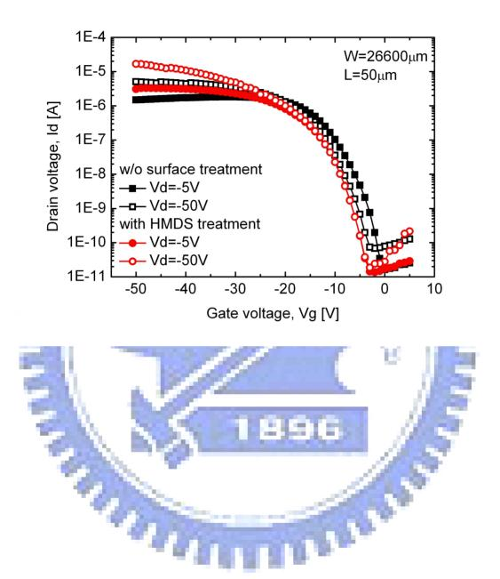
Figure 3.3.3-3 The Id-Vg electrical characteristics of pentacene TFTs with and without HMDS surface treatment. The channel width/length of devices are 26600/50  $\mu m/\mu m$ .
