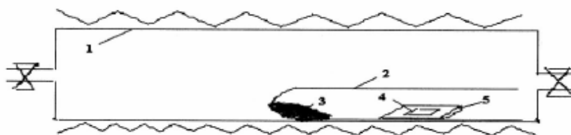
Figure 1-3. The schematic geometry of ZnO nanowires growth. 1. Furnace tube, 2. slender tube, 3. source, 4. template, 5. alumina supporter
