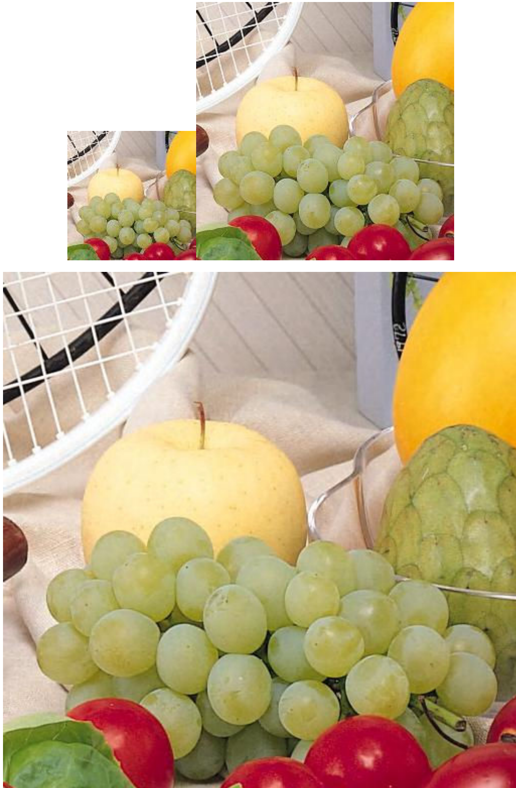
Figure 5-2 The decoded images of the resolution-based scalable media at different reconstruction levels with 5_3 filter
