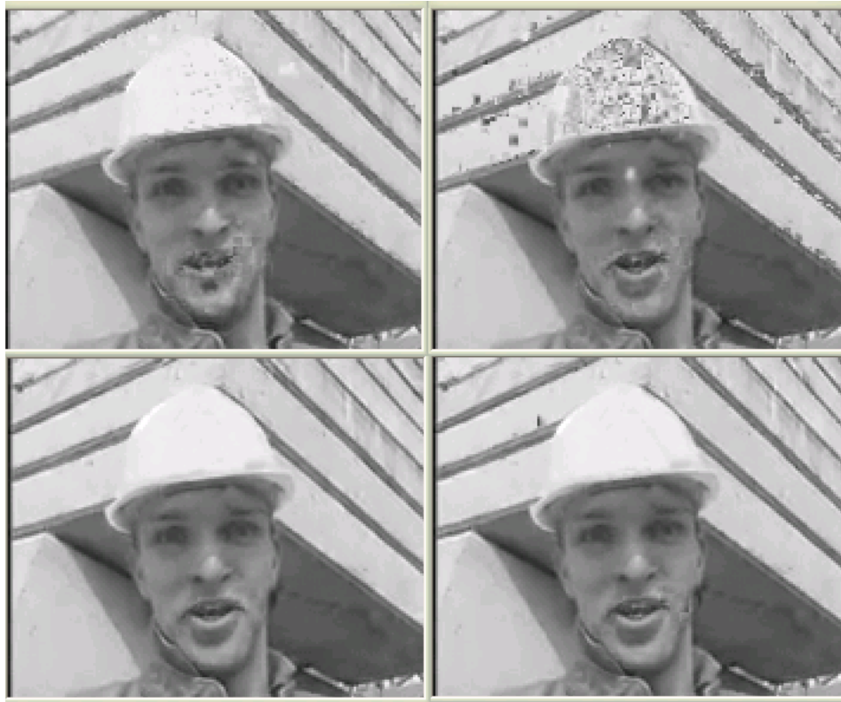
Fig. 4.22 Reconstructed frames based on FMP (top left), based on BMP (top right), based on BMP with full MV correction (bottom left), and based on BMP with partial MV correction (bottom right), (Foreman sequence, PLR 5.47%)
