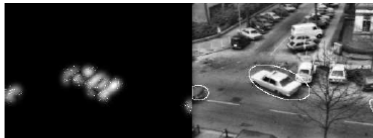
Figure 2-3 The example of detection result by applying Gabor Filters [5] Left figure is the detection results after applying Gabor filters, white particles represent the points used to clustering, and the right figure shows the final detection results.
