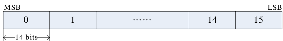
Fig. 26 Organization of a word in Luma SRAM
