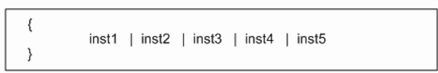
Figure 3.9: Syntax of instruction packet [3].
