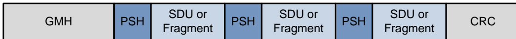
Figure 2-11: Examples of the Ordering of Payload and Subheaders in a MAC PDU
