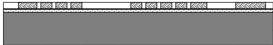
(b) The first copper plating for the coil part of the inductor.
