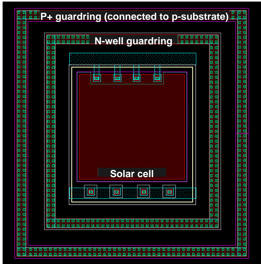
Figure 1.14. the top view of the layout of the single solar cell test key.
