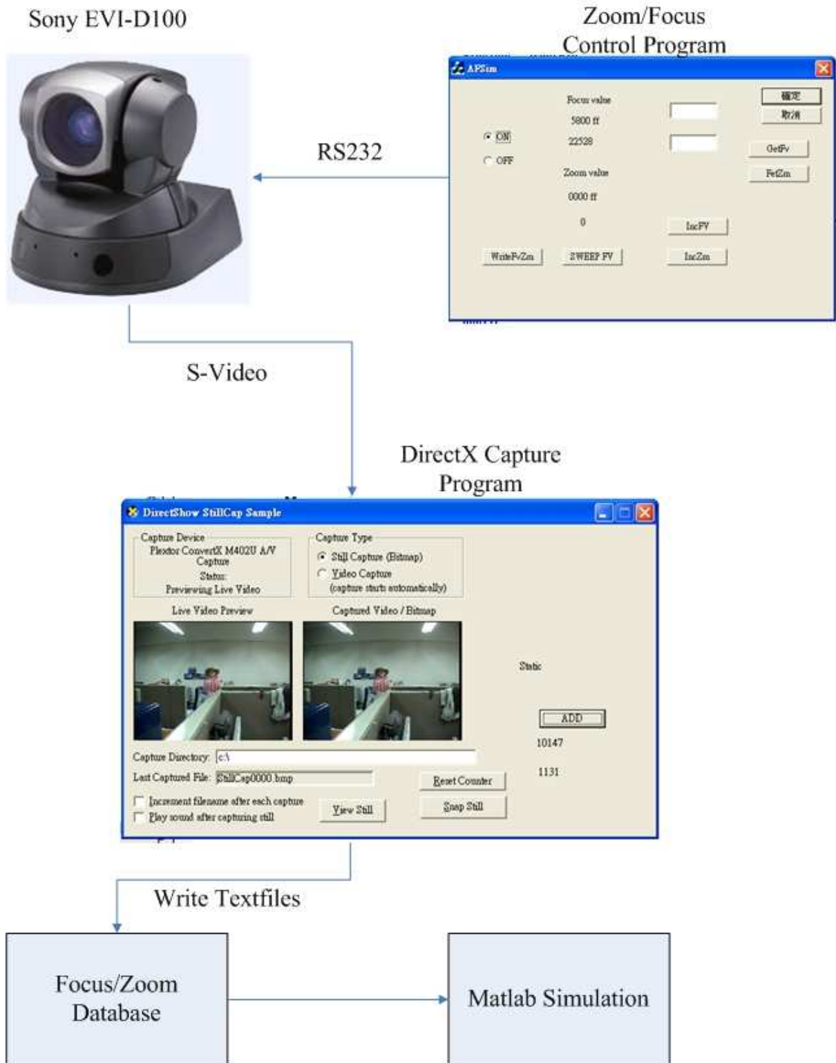
Figure 4.1 Block diagram of our auto-focusing system.
