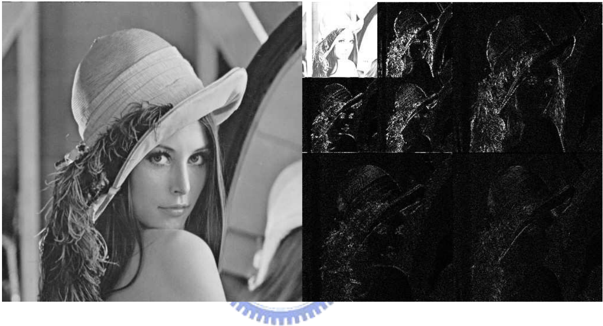
Figure 3.10 Original image and its wavelet transform.
