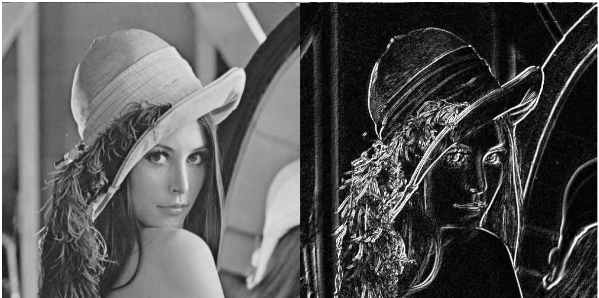
Figure 3.4 Original image and Sobel gradient.
